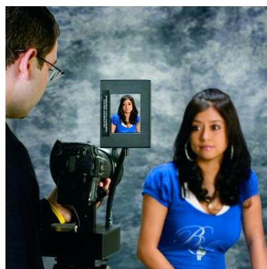
Large, 4.2" color LCD screen displays live view of the subject, captured image and camera data. The screen rotates from horizontal to vertical.
