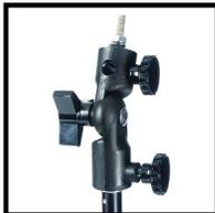
The R4108 Stand Adapter (812857) with locking teeth is used to mount our Battery Portable Lampheads on light stands. It includes an umbrella holder, continuous angle adjustment and 1/4"-20 threaded lamphead mount.
