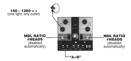
The "A" OUTPUT and "B" OUTPUT Dials are disabled automatically, and the modeling lamps track automatically with the POWER TRIM Dial.
