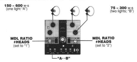
The modeling lamps track automatically with the flash settings via the two Dials ("A" and "B"). The POWER TRIM Dial varies the flash output over a 3-stop range, without affecting the lighting ratios nor the intensity of the modeling lamps.
